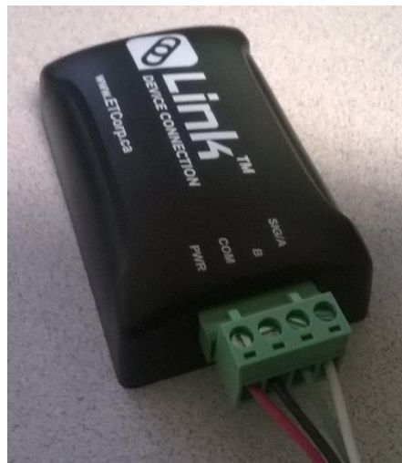
Figure 6 - USB to RS-485 Adapter Wiring using the Link
