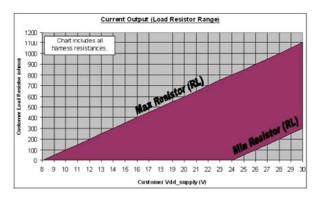
Min Resistor (RL) = 50 \* (Vdd - 24): for Vdd > 24VMax Resistor (RL) = 50 \* (Vdd - 8): for Vdd > 8V
